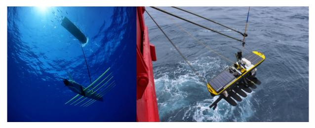
Figure 2. Left. The submerged portion of the wave glider. Right. A wave glider recovery from a surface craft.
