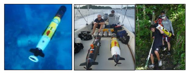
**Figure 1**. Left Panel: REMUS 100 passing over a sunken WWII aircraft; Center Panel: En route to a small boat deployment for two REMUS 100s and Right Panel: En route to a shore deployment of a REMUS 100.
