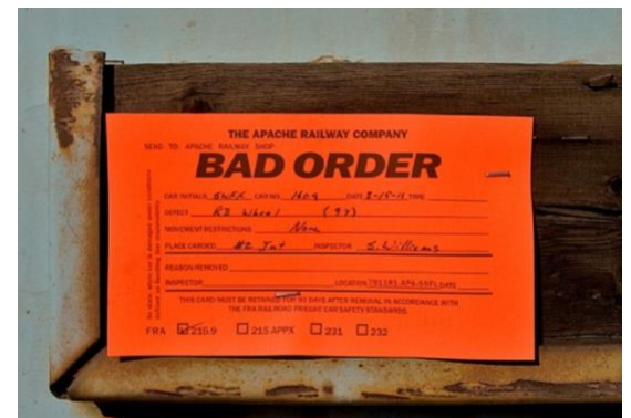
Figure 1 Example of a Bad Order tag that signifies a defect that must be fixed prior to being put back into service
