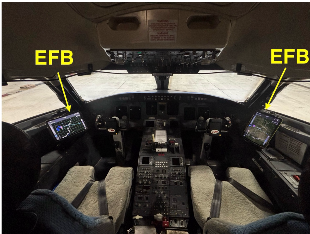
Figure 9. Electronic Flight Bag Mounted in CRJ700 Aircraft
