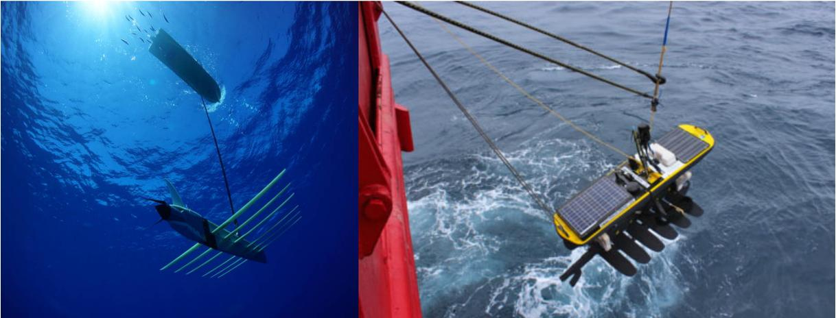
**Figure 2.** Left. The submerged portion of the wave glider. Right. A wave glider recovery from a surface craft.
