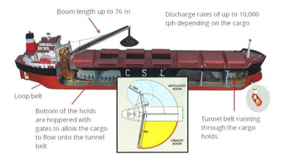
The graphic above highlights the very unique and environmentally friendly features of a typical self-unloading short sea ship.
