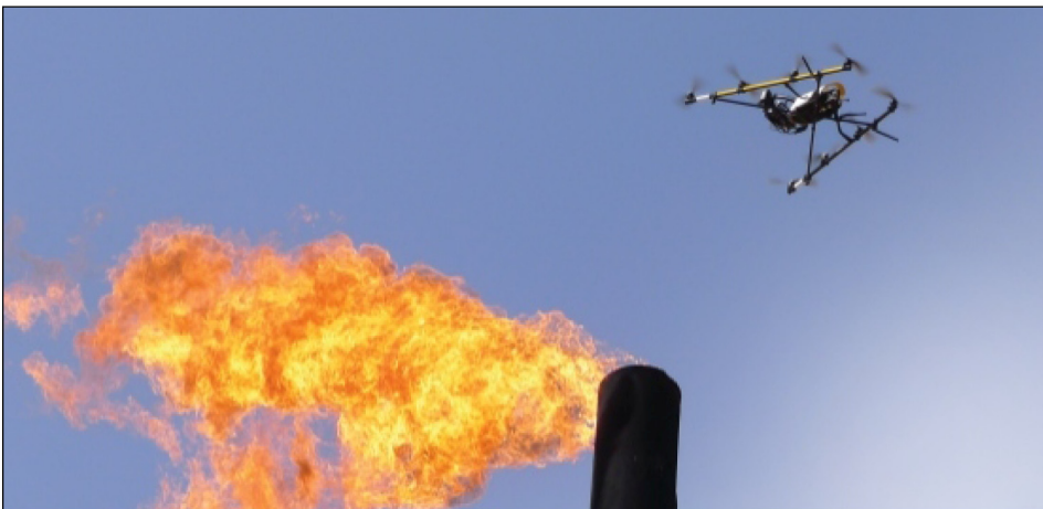
Flare stack inspection
